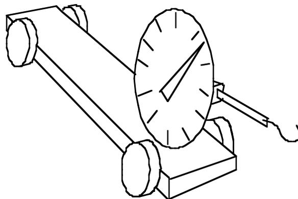
A very simple demonstration to use with the “spring balance cart” that should help students to begin thinking about the meaning of balanced and unbalanced forces is to hold the cart as a hanging mass extends the scale giving a reading as illustrated below:
