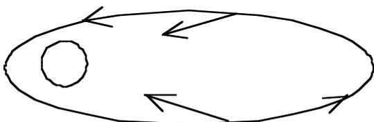
When the satellite is in the “top” part of its orbit and moving to the left, the force of gravity has a component in its direction of motion and thus speeds the satellite up. Likewise when the satellite is in the “bottom” part of its orbit and moving to the right, a component of the force of gravity is against its direction of motion, slowing it down.
