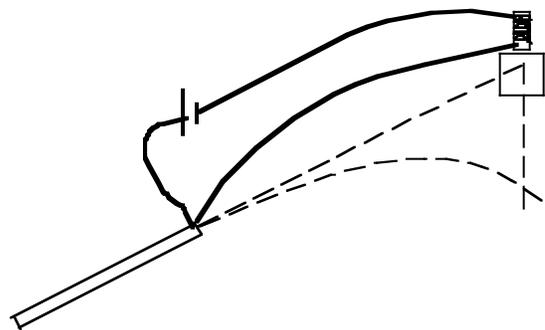
line path exactly the same distance that the “monkey” falls, insuring a hit. The apparatus can be challenging to get working properly but it is always rewarding.
