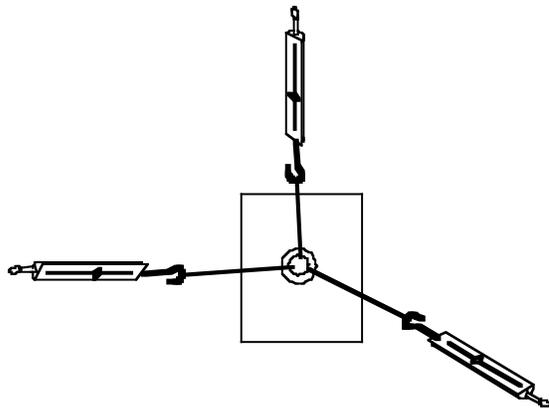
on the washer carefully holding a constant value while a fourth student sketches the position of the center of the washer, the direction the strings are pulling and writes on each string drawing the reading on each of the spring balances. This “data sketch” can now be used to construct the force vectors involved and test to see if they sum to zero. Other string and spring balance configurations can be easily repeated on a separate piece of paper.
