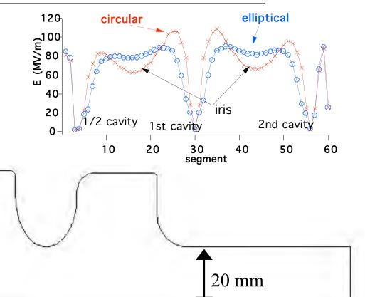
$F_r = 3.003 \text{ GHz}$   $R_s = 6 \text{ M}\Omega$ Q = 14530
