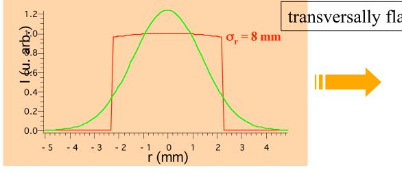
transversally flat, longitudinal profile is gaussian
