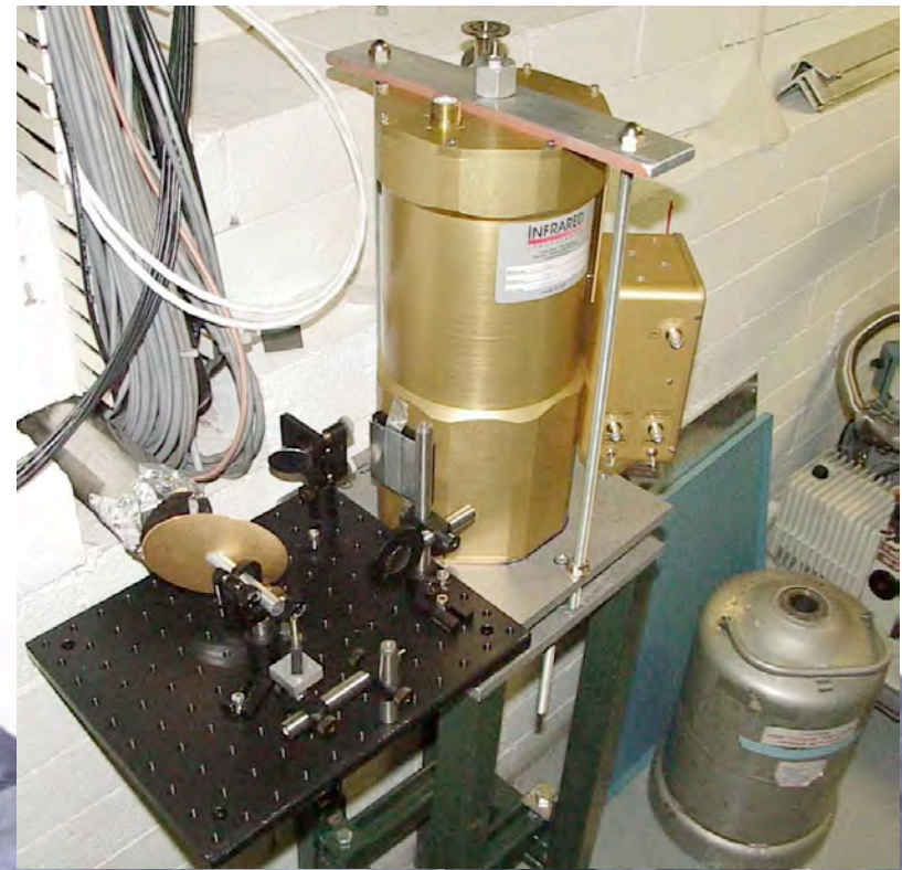
Brookhaven Si Bolometer for CER detection.[1]
