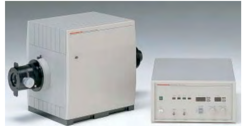
Hamamatsu "FESCA-200" (Femtosecond Streak Camera). Temporal resolution: 200 fs.
