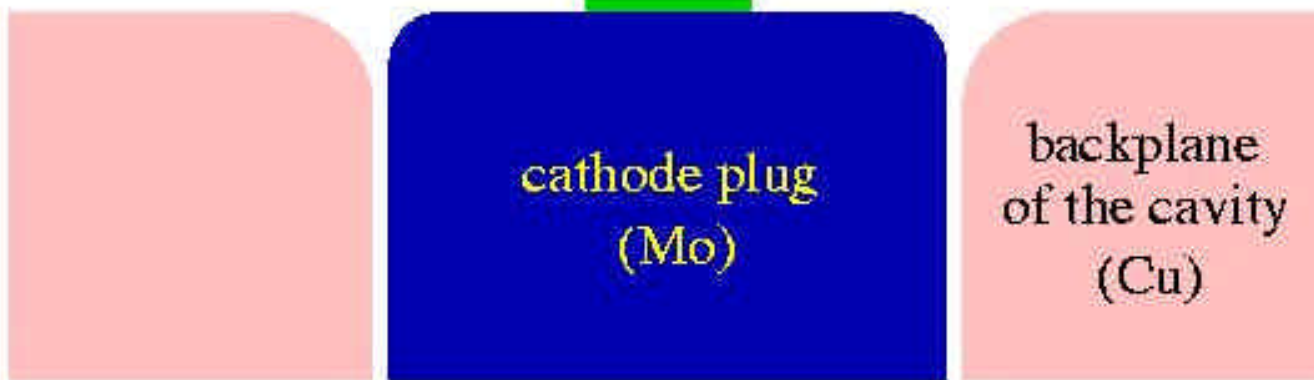
Schematic cross section of the cathode and the backplane of the Cu cavity
