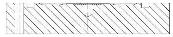
Flat shape of the cathode was changed to compensate the effect of the RF seal on the half cell frequency
