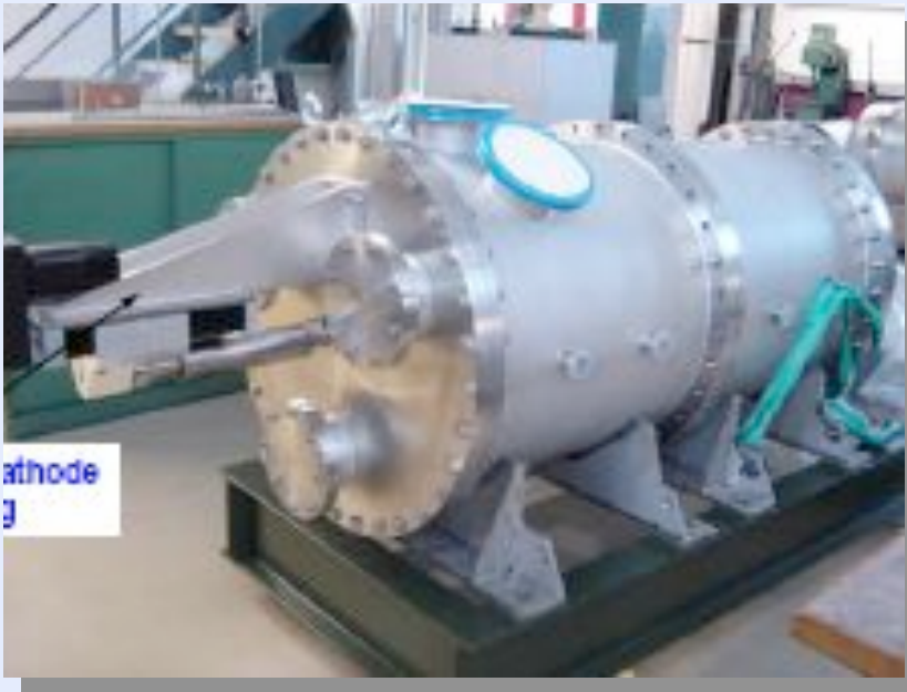
High Voltage Pulser ( under assembly !) Air Core Transformer Technology
