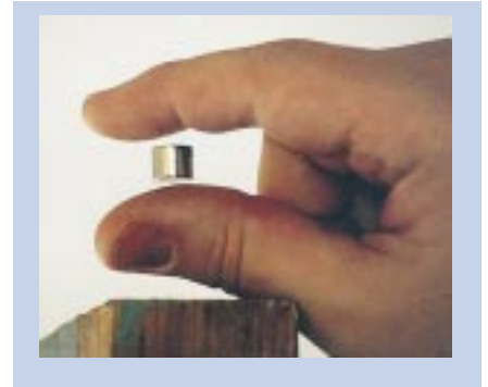
Figure 2 Levitation at your fingertips. A strong NdFeB magnet (1.4 tesla) levitates 2.5 metres below a powerful superconducting magnet. The field at the levitation point is about 500 Gauss.
