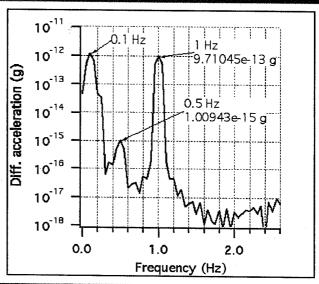
Simulation results for realistic error at release and construction imperfections
