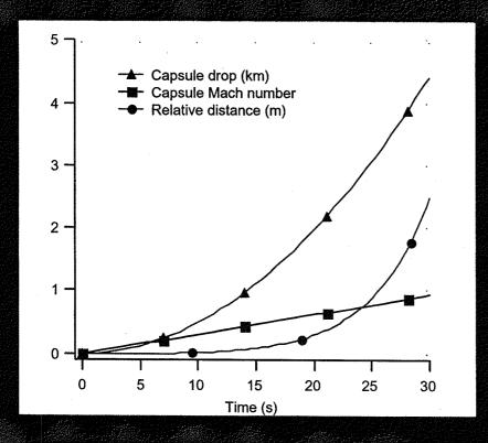
Expected free-fall characteristics of experiment for a capsule mass of 1700 kg
