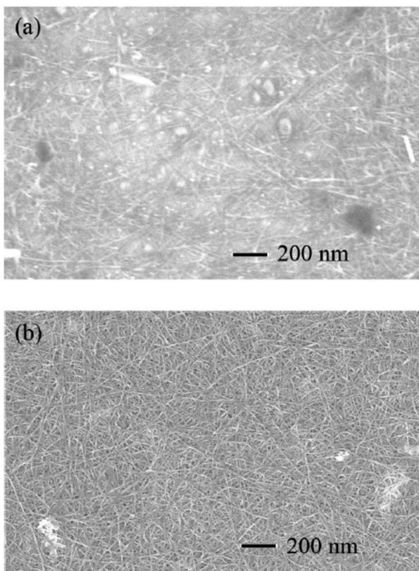
FIG. 1. SEM of two SWCNT network samples with different densities: (a) submonolayer nanotube film and (b) nanotube film with thickness of about 20 nm.
