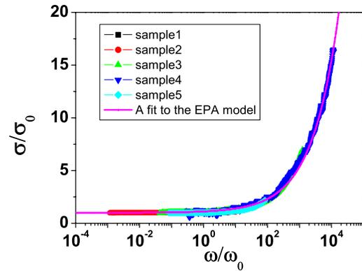
FIG. 4. (Color online) Master scaling curve showing the ac conductance for SWCNT network samples (spray method) with different densities at room temperature. The red (gray) solid line is a fit to the extended pair approximation model  $k=0.12$  and  $s=0.52$ .
