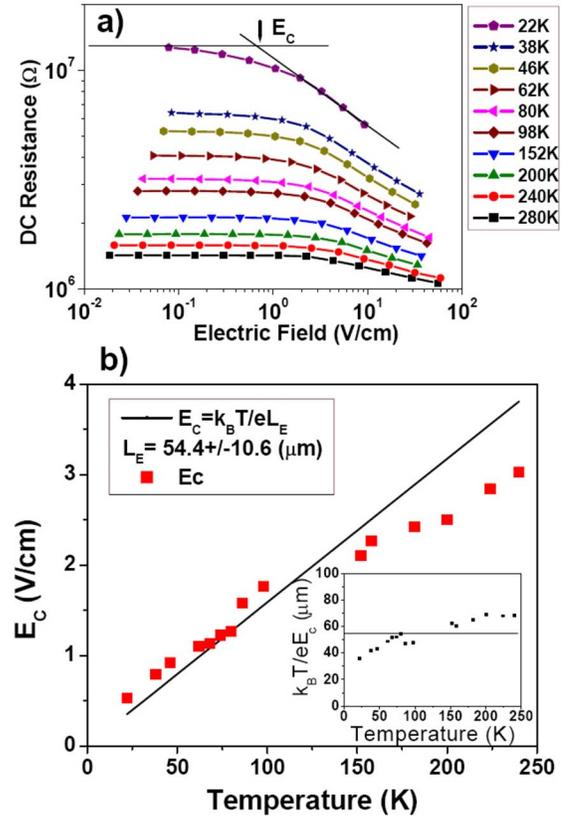
FIG. 5. (Color online) (a) dc resistance vs electric field for a submonolayer (sample 5) SWCNT network at different temperatures. (b)  $E_c$  vs temperature and extracted length scale for this sample.
