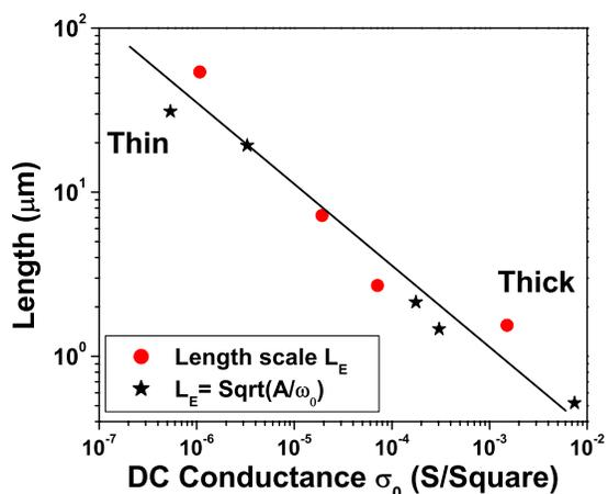
FIG. 6. (Color online) Comparison of the length scale  $L_E$  obtained from electric-field-dependent dc conductance data (red dot) and the estimated length scale from frequency-dependent conductance measurement  $\sqrt{A/\omega_0}$  (black star) of SWCNT networks of various densities. The line has slope  $-1/2$  in the log-log plot.
