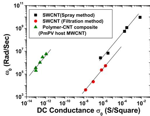
FIG. 3. (Color online) The onset frequency vs dc conductance for different SWCNT networks at room temperature. The three solid lines all have a slope of 1.
