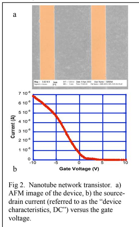
Fig 2. Nanotube network transistor. a) AFM image of the device, b) the source-drain current (referred to as the “device characteristics, DC”) versus the gate voltage.
