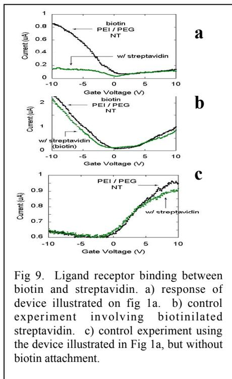
Fig 9. Ligand receptor binding between biotin and streptavidin. a) response of device illustrated on fig 1a. b) control experiment involving biotinylated streptavidin. c) control experiment using the device illustrated in Fig 1a, but without biotin attachment.
