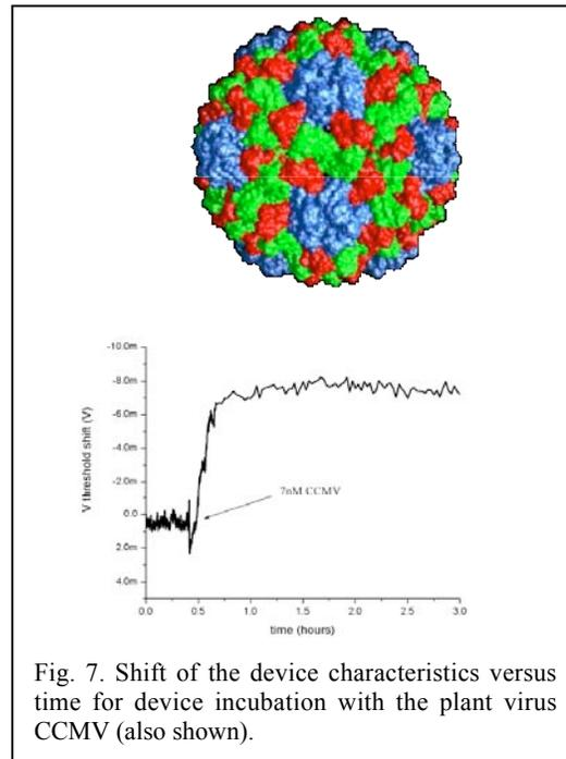
Fig. 7. Shift of the device characteristics versus time for device incubation with the plant virus CCMV (also shown).
