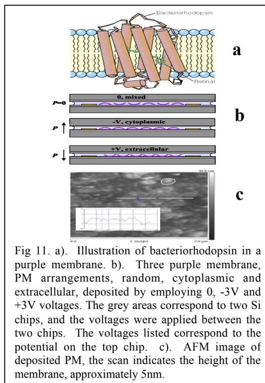
Fig 11. a). Illustration of bacteriorhodopsin in a purple membrane. b). Three purple membrane, PM arrangements, random, cytoplasmic and extracellular, deposited by employing 0, -3V and +3V voltages. The grey areas correspond to two Si chips, and the voltages were applied between the two chips. The voltages listed correspond to the potential on the top chip. c). AFM image of deposited PM, the scan indicates the height of the membrane, approximately 5nm.
