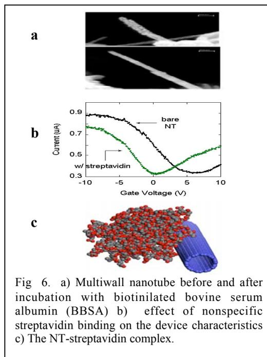
Fig 6. a) Multiwall nanotube before and after incubation with biotinylated bovine serum albumin (BBSA) b) effect of nonspecific streptavidin binding on the device characteristics c) The NT-streptavidin complex.
