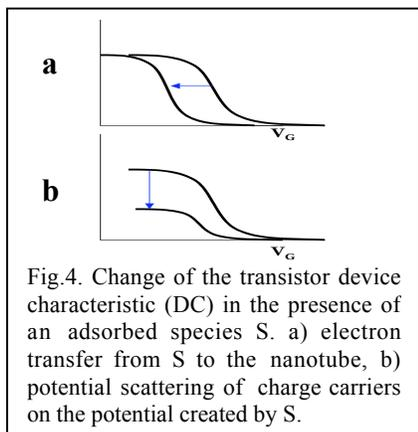
Fig.4. Change of the transistor device characteristic (DC) in the presence of an adsorbed species S. a) electron transfer from S to the nanotube, b) potential scattering of charge carriers on the potential created by S.
