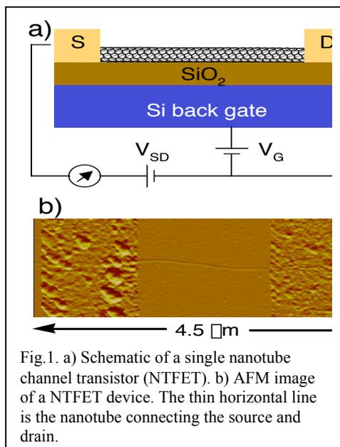
Fig.1. a) Schematic of a single nanotube channel transistor (NTFET). b) AFM image of a NTFET device. The thin horizontal line is the nanotube connecting the source and drain.
