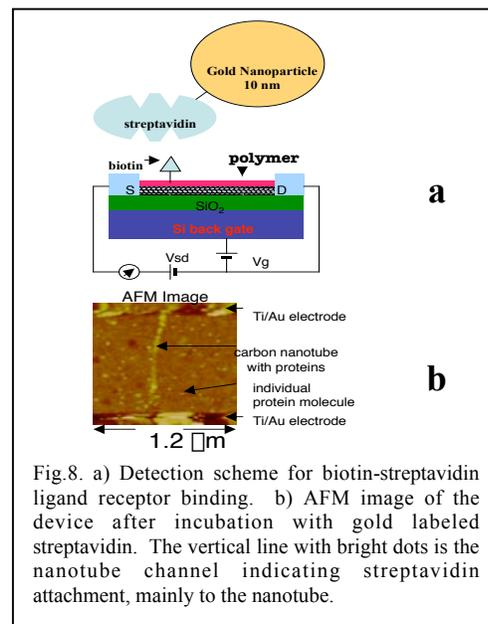
Fig.8. a) Detection scheme for biotin-streptavidin ligand receptor binding. b) AFM image of the device after incubation with gold labeled streptavidin. The vertical line with bright dots is the nanotube channel indicating streptavidin attachment, mainly to the nanotube.
