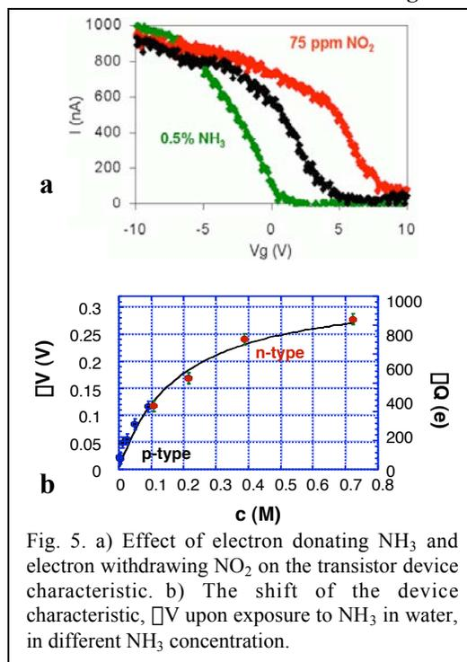
Fig. 5. a) Effect of electron donating  $\text{NH}_3$  and electron withdrawing  $\text{NO}_2$  on the transistor device characteristic. b) The shift of the device characteristic,  $\Delta V$  upon exposure to  $\text{NH}_3$  in water, in different  $\text{NH}_3$  concentration.
