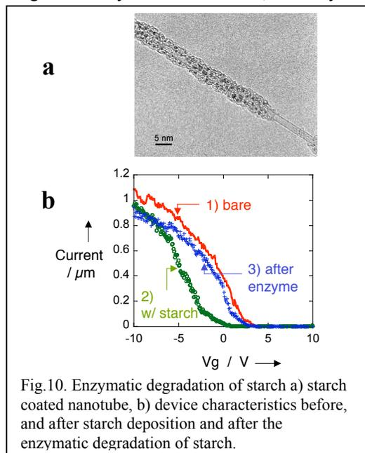
Fig.10. Enzymatic degradation of starch a) starch coated nanotube, b) device characteristics before, and after starch deposition and after the enzymatic degradation of starch.
