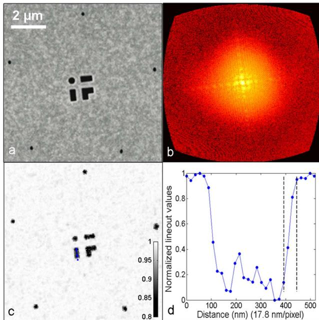
Fig. 3. (Color online) (a) SEM image of the sample. (b) Log of the curvature corrected hologram used in the iterative phase retrieval ( $q_{\max} = \pm 0.211 \text{ nm}^{-1}$ ). (c) Reconstructed image of the sample using a phase-retrieval algorithm to refine the resolution to 53 nm (17.8 nm per pixel), as demonstrated in the lineout (dotted line) shown in (d).
