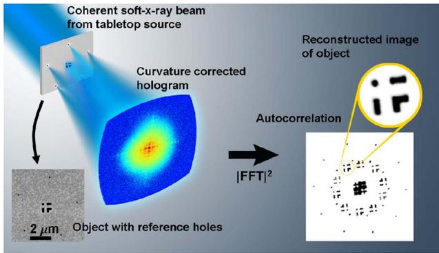
Fig. 1. (Color online) Multiple reference FT holography. A coherent high-harmonic beam with  $\lambda=29$  nm illuminates a test pattern surrounded by five reference holes. The scattered light interferes and is recorded on a CCD camera in the far field as a hologram (log scale). The spatial autocorrelation of the object can be retrieved by taking the squared magnitude of the Fourier transform of the hologram. A single subimage from the autocorrelation is shown.
