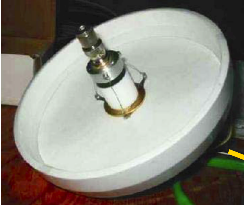
UV LED Light Source (15cm \phi )
