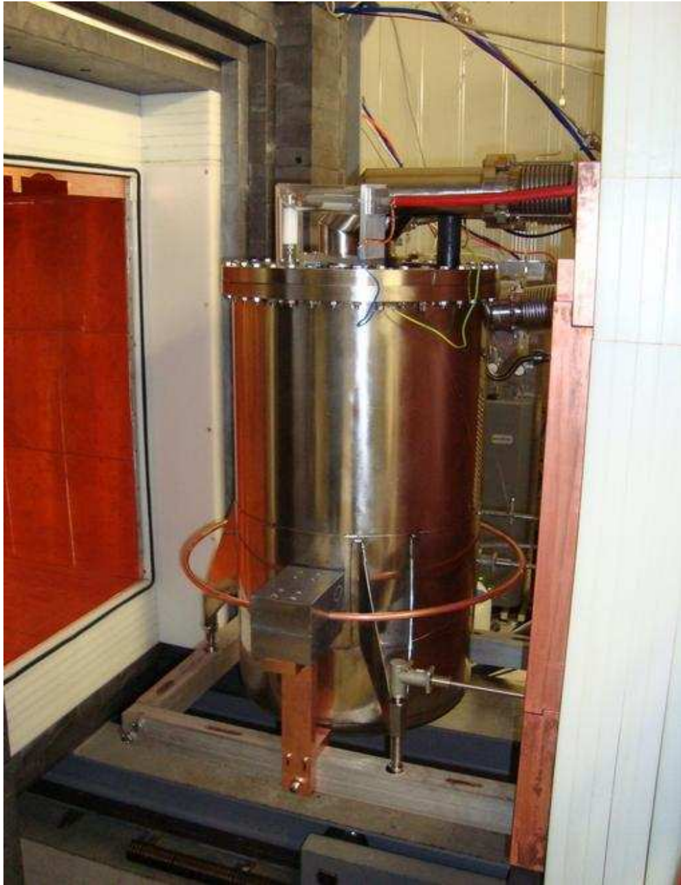
Figure 5.13: A picture of the XENON100 detector outside of the shielding. The copper tube encircling the detector is used to introduce calibration sources, and the lead shield surrounding part of the copper tube is used to stop \gamma -rays from the AmBe neutron source.
