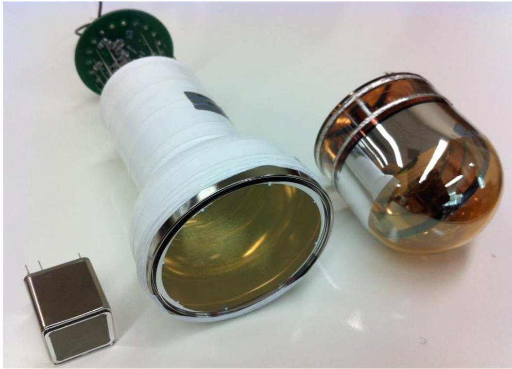
Figure 8.2: A comparison between a Hamamatsu R8520 1" PMT (left), a Hamamatsu R11065 3" PMT (center) and the QUPID (right). The R8520 is currently being used in the XENON100 detector, while the R11065 and QUPID are candidates for future dark matter detectors.
