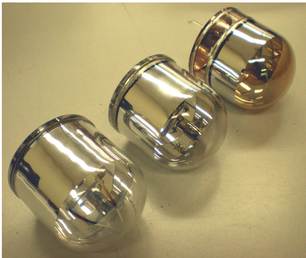
Figure 8.3: A comparison between old versions of the QUPID and the current version. Note that the new version (top-right) has an intermediate quartz ring and a small quartz pipe, while the old versions do not.
