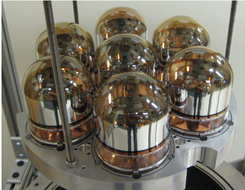
Figure 9.3: The support for the 7-QUPID system, with seven QUPIDs installed in their individual holders. Here, the individual holders and the 7-QUPID support are made of aluminum for ease of machining. The version that will be used in future dark matter detectors will be made of OFHC copper.
