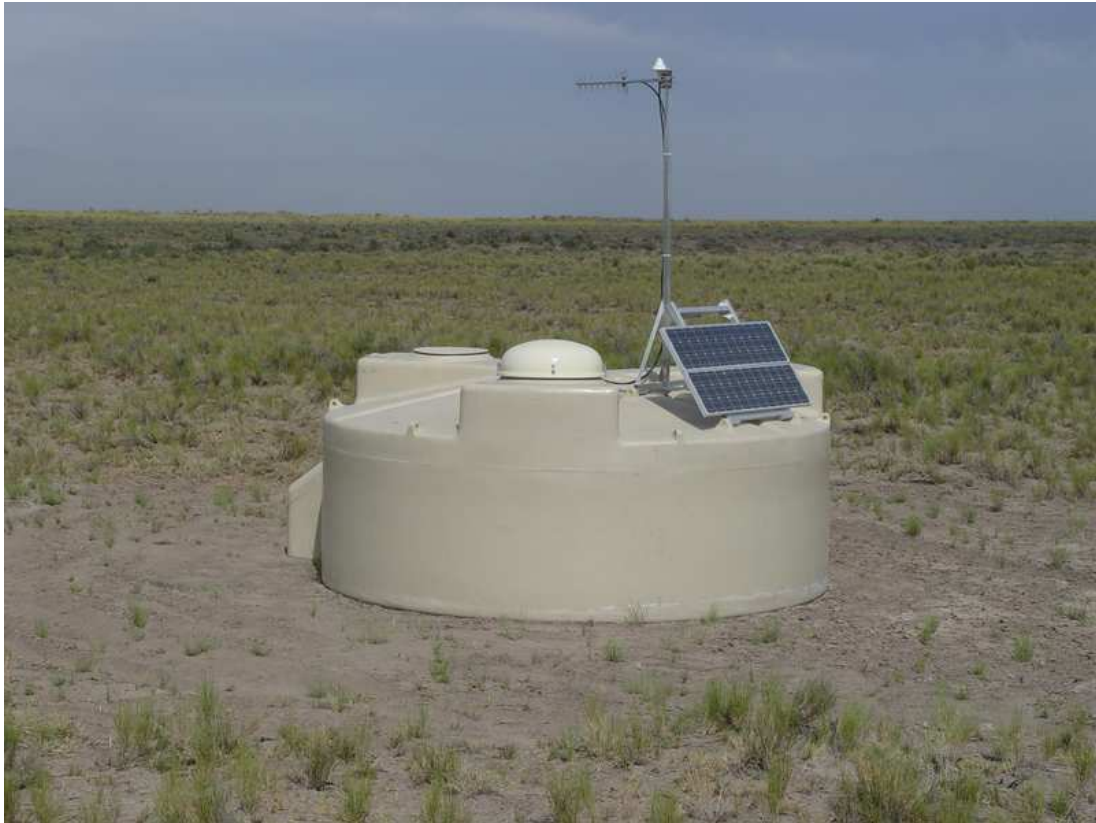
Figure 3.5: A picture of a water Cherenkov detector deployed in the Pampa Amarilla in Argentina. The beige dome contains all the electronics of the station and the panel mounted on the top of the station is the solar panel. The antenna for the wireless communications system can also be seen as well as the GPS antenna mounted on top of the antenna mast. Three “propellers” can be seen, one with the beige dome on top, where the PMTs are housed.
