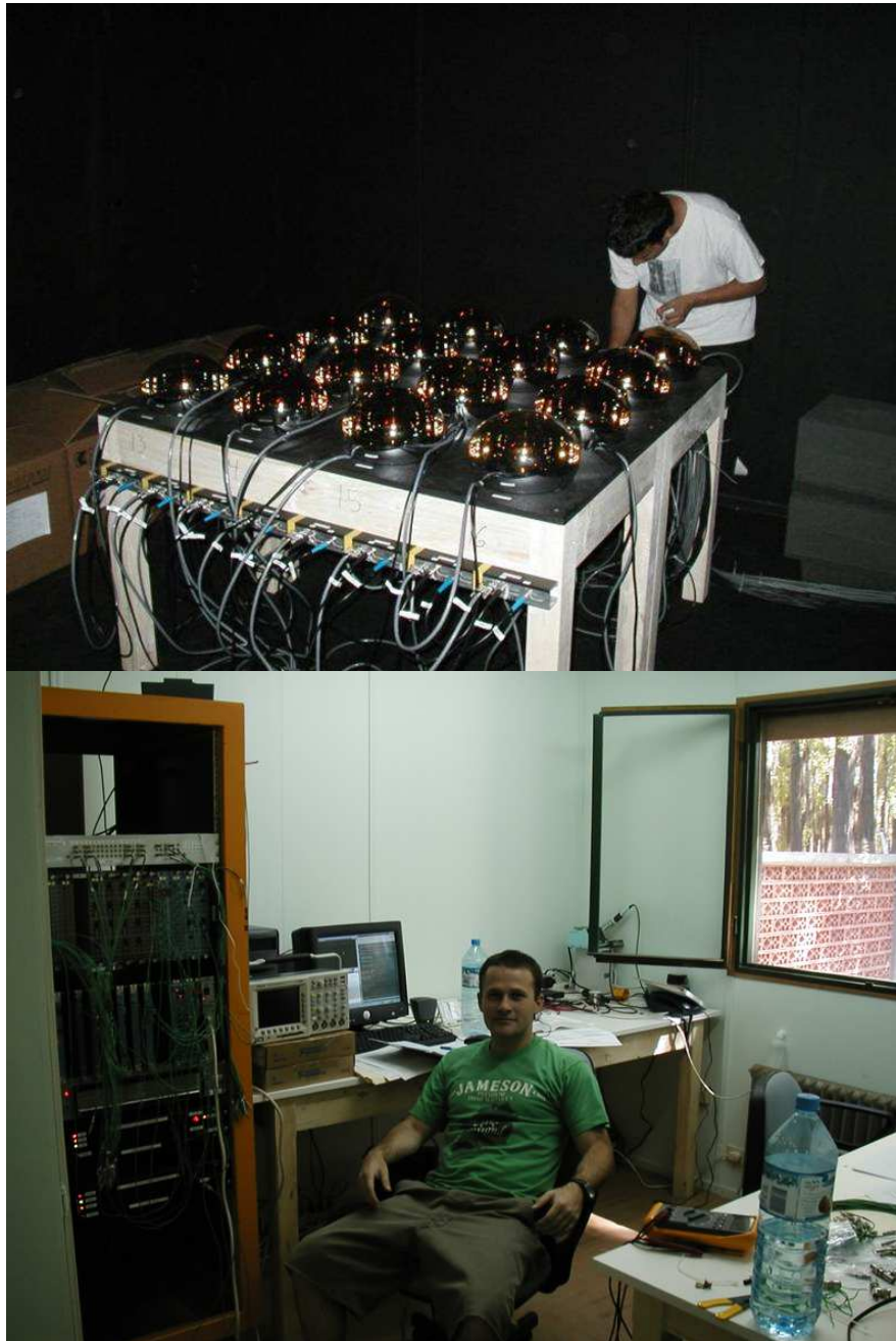
Figure 4.7: Top: PMTs in the dark room. Bottom: The DAQ setup with the CAMAC crate and custom electronics in the rack on the left.
