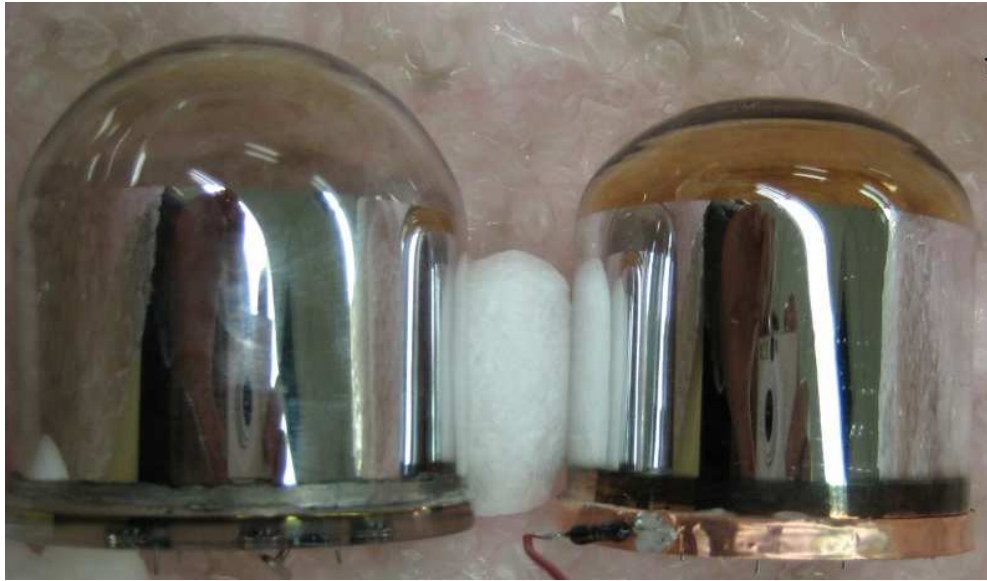
Figure 6.23: Comparison of a normal mechanical sample (left) and the first working version of the QUPID (right) that was not constructed to specification
