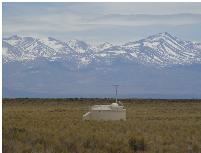
Figure 3.3: A surface detector station on the Pampa. Note the attached components, antenna, solar panels, etc. The photo-tubes and water are contained inside the plastic shell.
