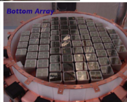
Figure 3.2: Top: The Time Projection Chamber (TPC). Bottom: The top and bottom PMT arrays.
