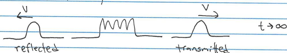
Scattering theory answers the question of how much of the initial wave packet, i.e., how much probability amplitude, is reflected and how much is transmitted.
