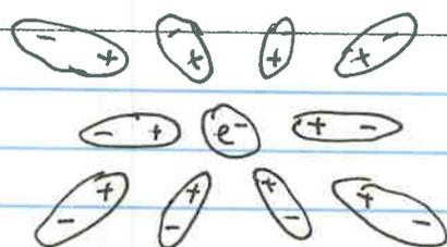
Here, I have denoted  $e^+e^-$  pairs by the plobs with + and - inside. These virtual particles effectively screen the electric charge of the electron making it appear smaller when you are a further distance away. In ~~the~~ turn, it appears that  $\alpha$  is smaller when you are further away!
