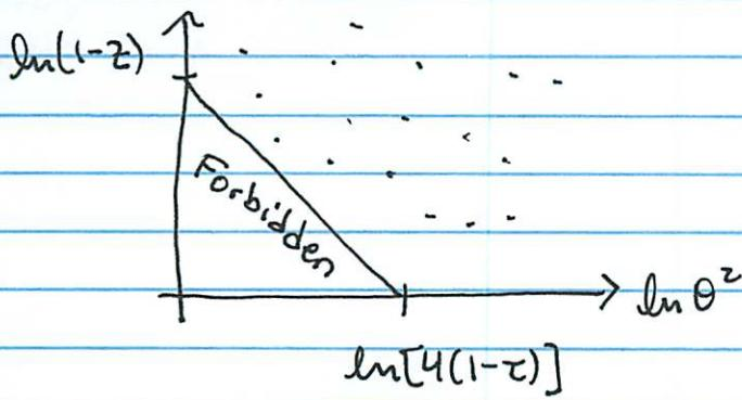
To determine the probability that no gluon emissions land in the triangle, we imagine breaking it up into tiny pieces and forbidding any emission in each of the pieces.
