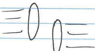
Protons are Lorentz contracted into pancake shapes from their spherical shape at rest.
