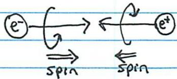
In this configuration, the spins of the  $e^+$  and  $e^-$  are in opposite directions, which sum to 0 spin! This spin configuration is not allowed. Therefore, for production of a spin-1 photon we must align the spins of  $e^+$  and  $e^-$ :
