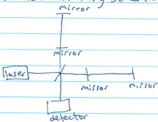
A laser sends coherent light to a half-silvered mirror. That light is then split to two perpendicular arms which are each about 4 km long and are the purest vacuums in the universe. The light in the arms bounces back and forth hundreds of times before being recombined in a detector.
